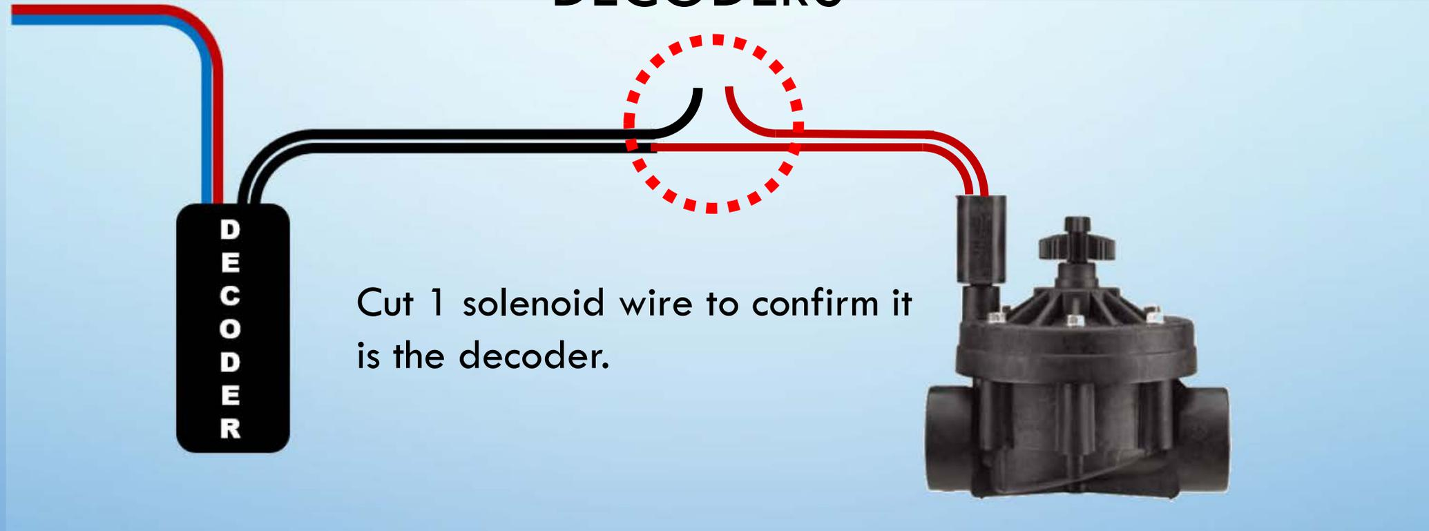
Cut 1 solenoid wire to confirm it is the decoder.
